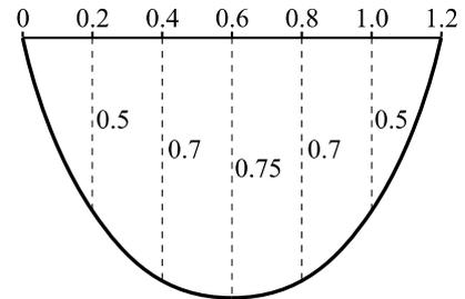
$$\text{Cross sectional area} \doteq \frac{h}{2} \times 6.3 = \frac{0.2}{2} \times 6.3 = 0.63 \text{ m}^2$$
