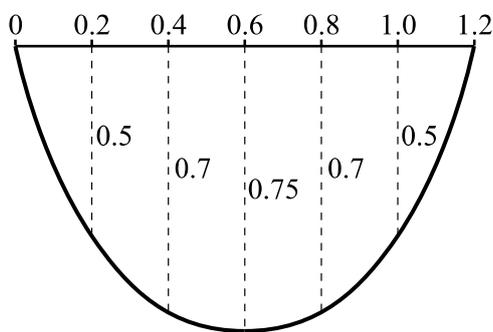
The diagram above shows the cross-section of one ditch, with measurements in metres. The width of the ditch is 1.2 m
